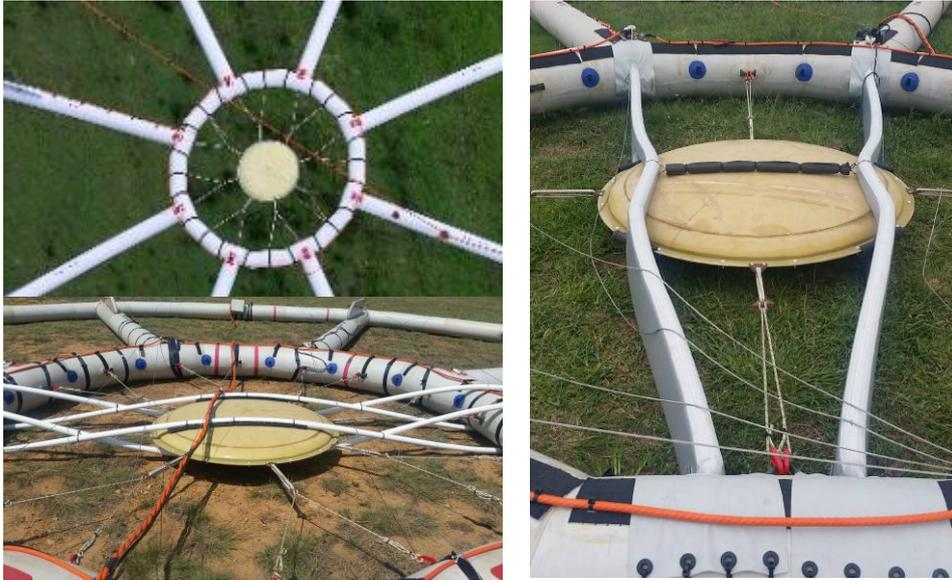
Figure 2: Receiver suspension improvements. Top left: Bungees only. Bottom left: Bungees and PVC pipes. Right: Bungees and inflatable support beams.
